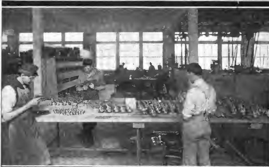
Part of the Space Devoted to Testing, Showing Lots of Model L & F Carbureters Undergoing Final Inspection
